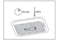
Remove the spray head from the ultrasonic bath and rinse with demineralised water;
