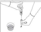
Using a disposable syringe (25 ml vol.) inject the demineralised water into the spray head cavity for at least 5 times in order to eliminate any detergent residue;
