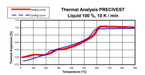
By using the Non Precious metal to ceramic alloys, we suggest you to mix 80% of the High Expansion liquid 931-2000, with 20% distilled Water which increases 0,5% the setting expansion, and which is equivalent to 100% of the normal standard liquid.
